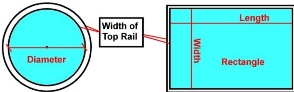
2-B. If you have an Oval pool, we need the overall Length of the pool, Width of the pool ("water to water") and the Width of the top rail. We also need a set of dimensions that will allow us to fabricate the exact cover for your pool.
