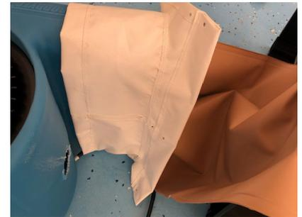
6. Slide the white boot over the snorkel tube and the snout of the blower so that it rests firmly up against the blower housing. You may have to tug on it a bit to get it into place.
