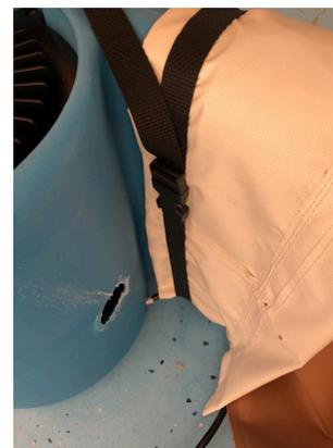
9. Snap the buckle and pull the black strap tightly. (If you are not able to tension the strap, it is looped incorrectly through the buckle. Try again!) Turn the blower power switch to the "ON" position and set the speed to the "High" setting (if you have a residential dome, the pressure switch will automatically turn the blower on and off as needed).
