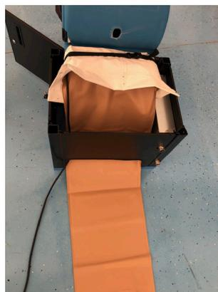
10. Slide the end of the snorkel tube down through the discharge port of the Dome Heater housing and lower the blower into the hole.
