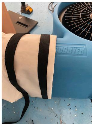
8. Use the black strap and buckle provided to fully wrap around the boot/snorkel tube/ and snout. The buckle on the strap can be a bit tricky (see #9).
